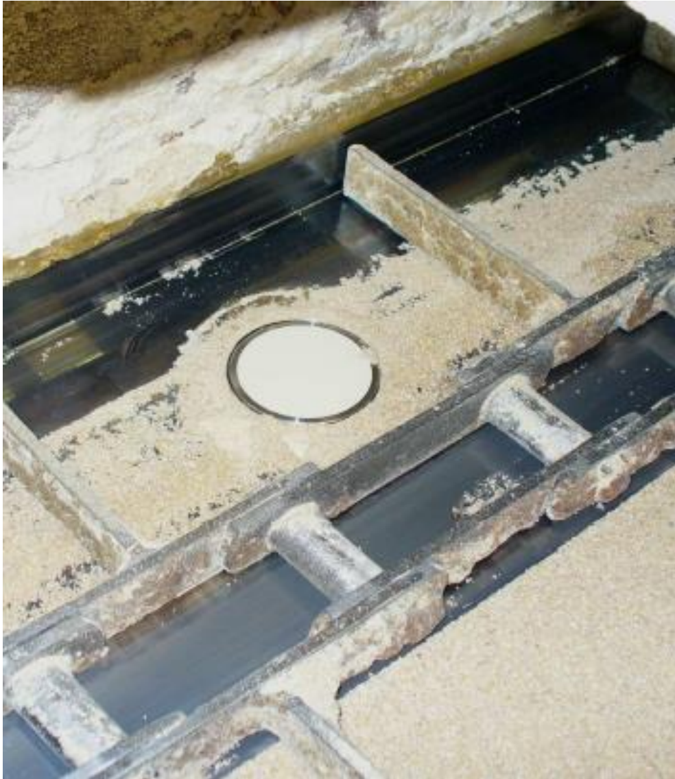
Humy mounted on the floor of the chain conveyor
