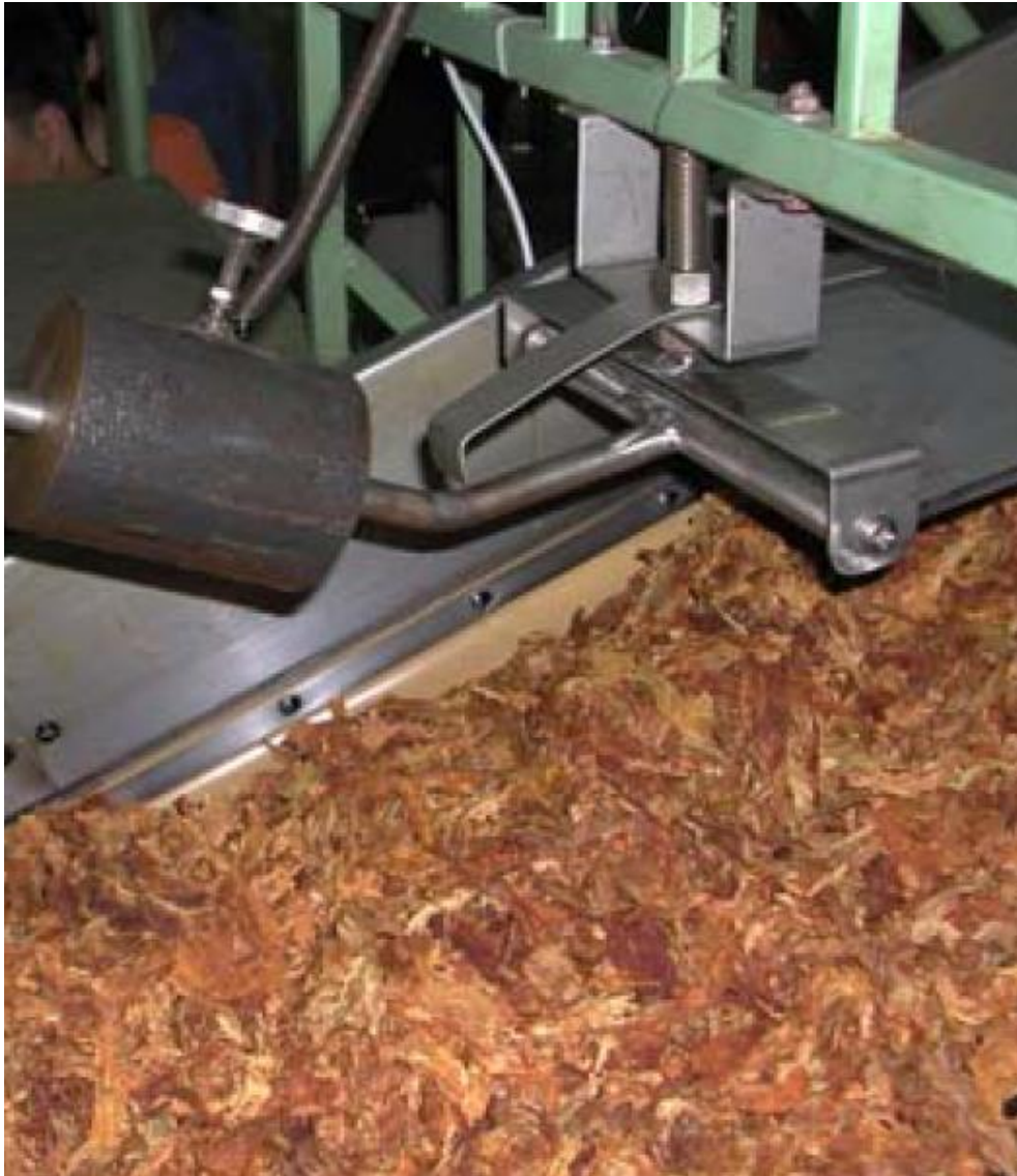
Humy 3000 installed on top of the conveyor belt
