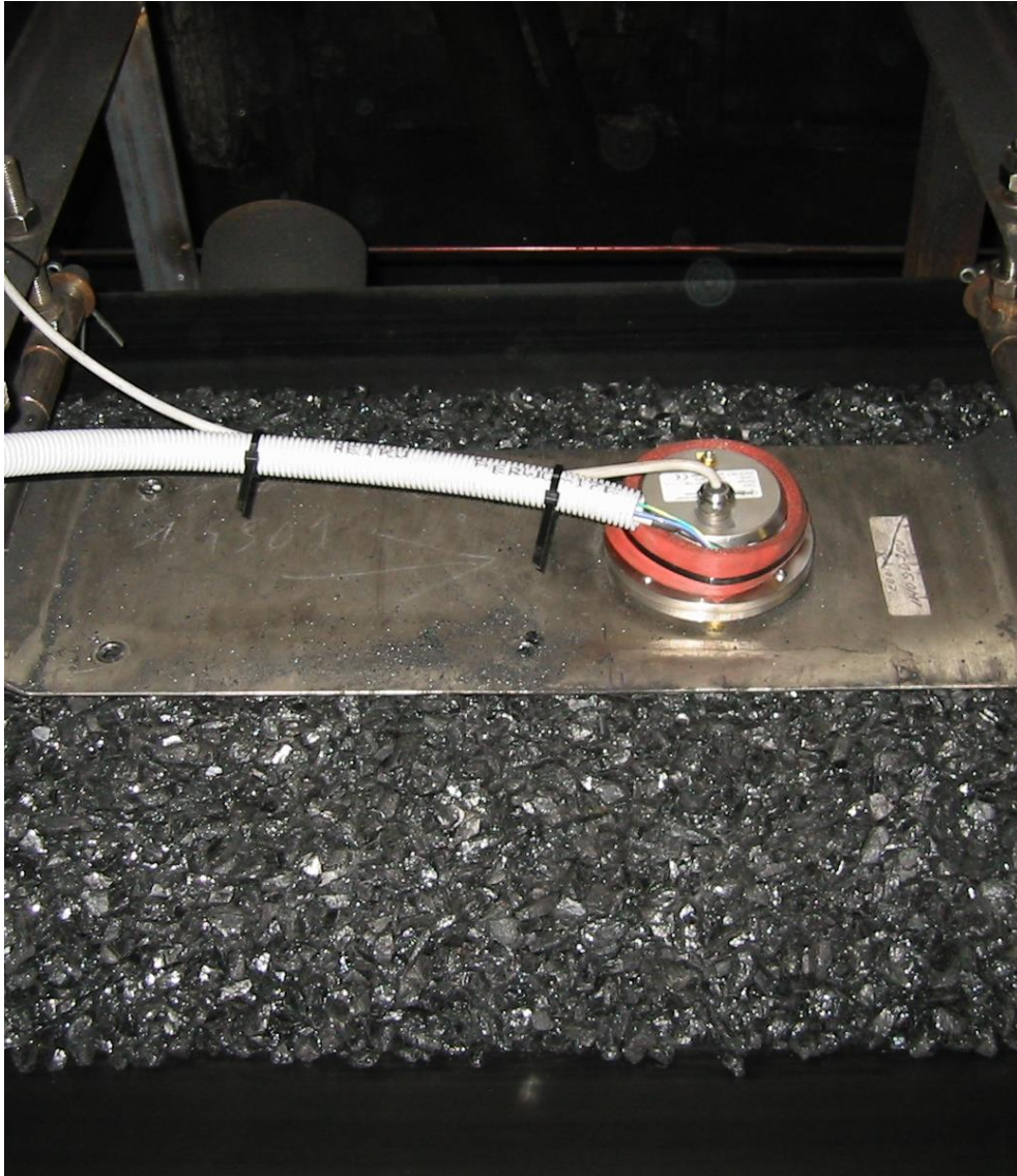
A Humy sensor measures the moisture of coal
