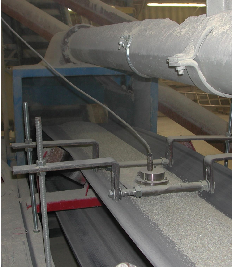
A Humy is installed at BASF on a conveyor belt
