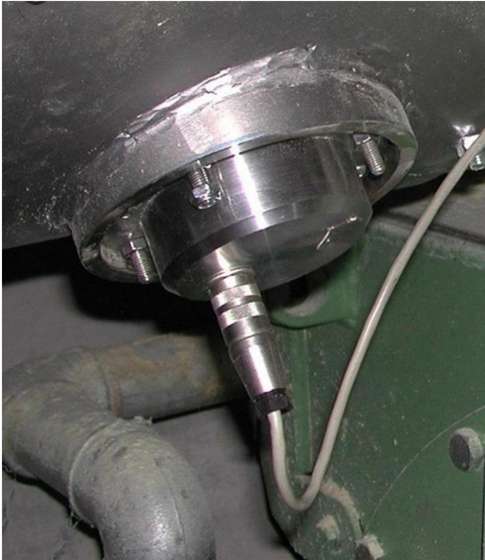
Humy 3000 installed in a screw conveyor
