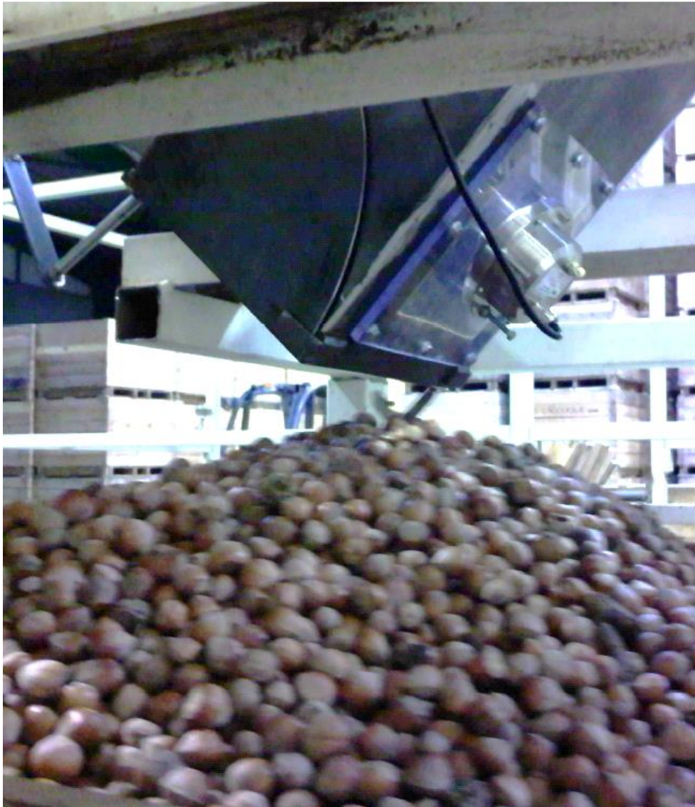
A Humy is measuring the moisture of the nuts
