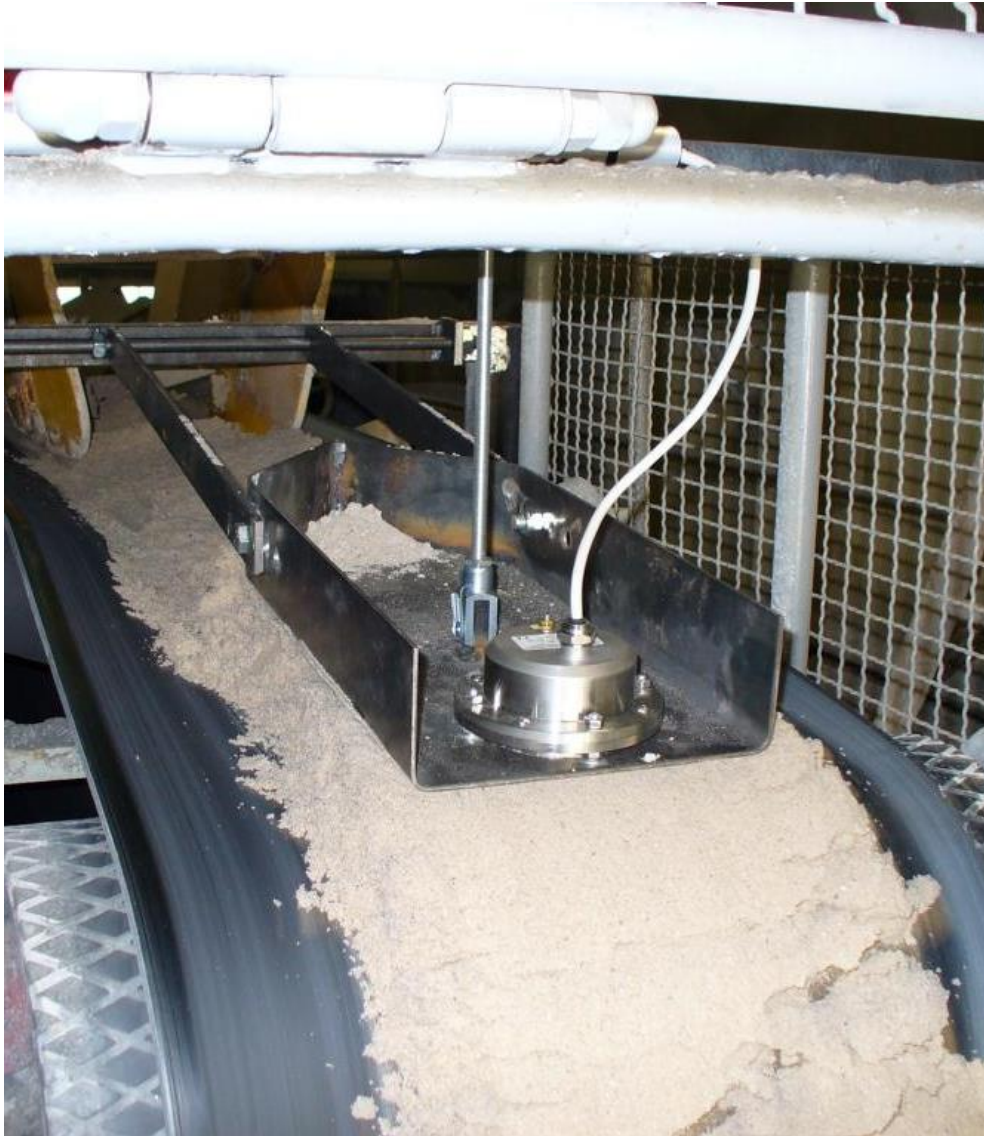
A Humy 3000 measures the raw sand on the conveyor belt
