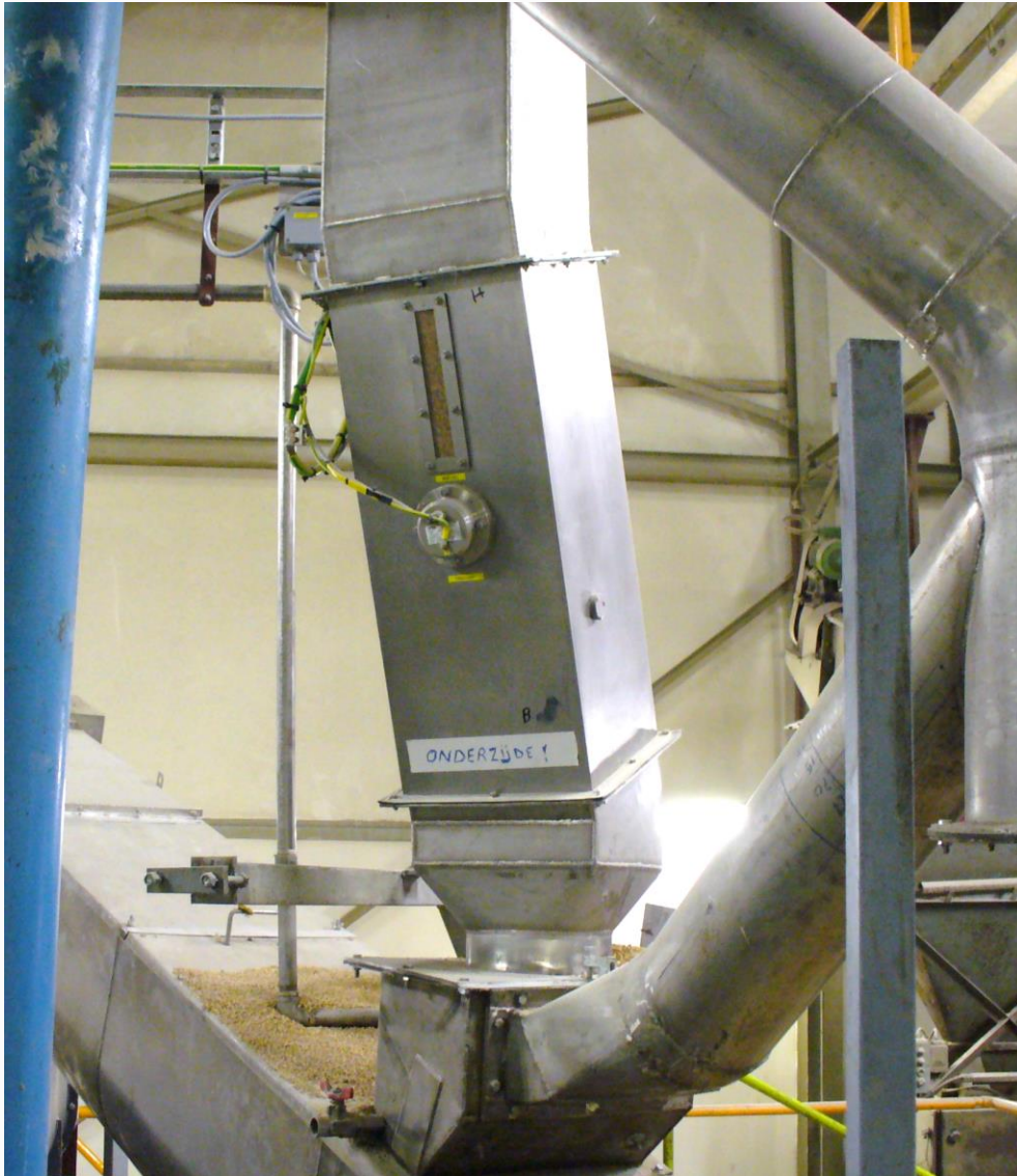
Optimal measuring spot in a fill-level regulated hopper
