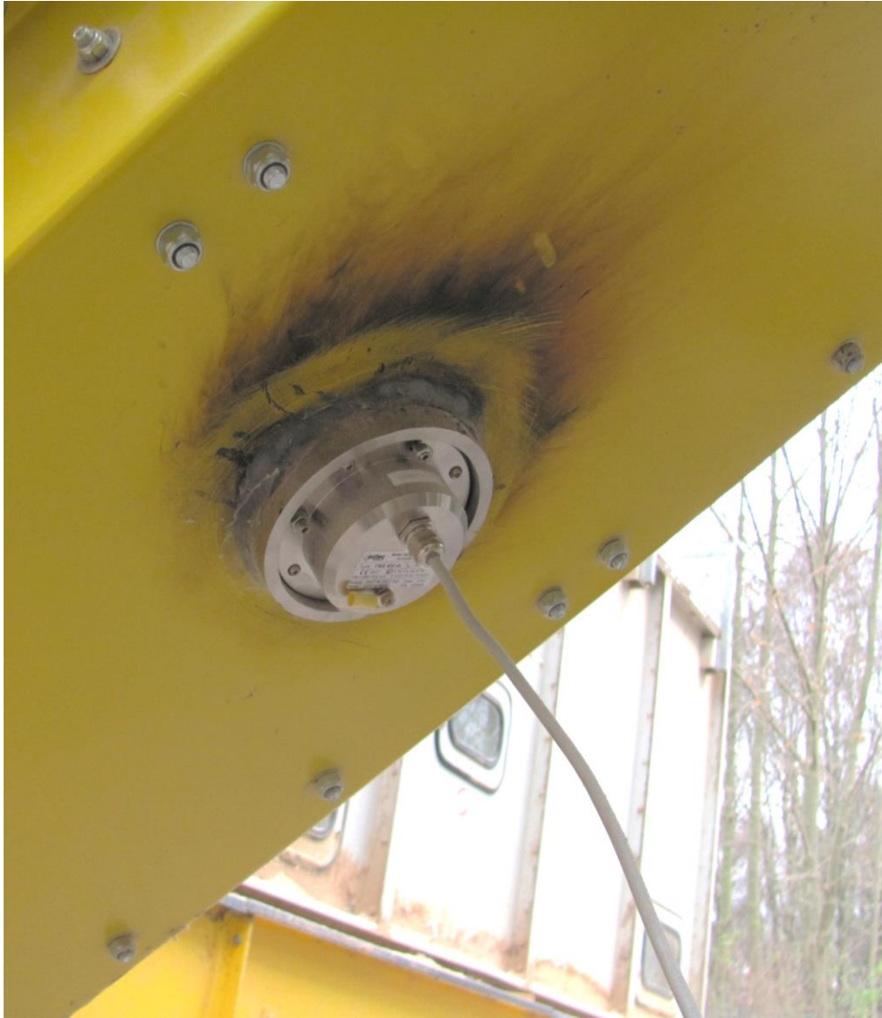
Humy 3000 installed in a trough chain conveyor
