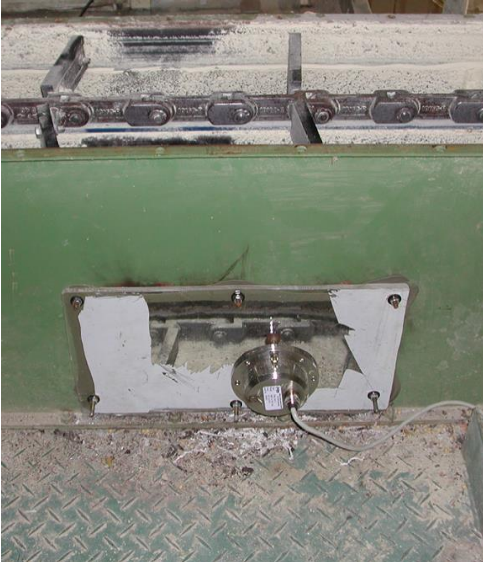
Humy installed at the side of a chain conveyor
