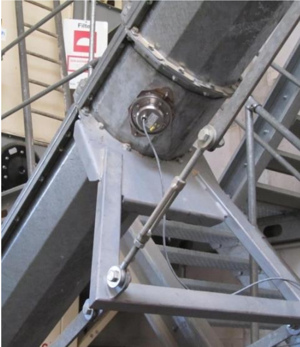
Humy 3000 installed in a trough chain conveyor
