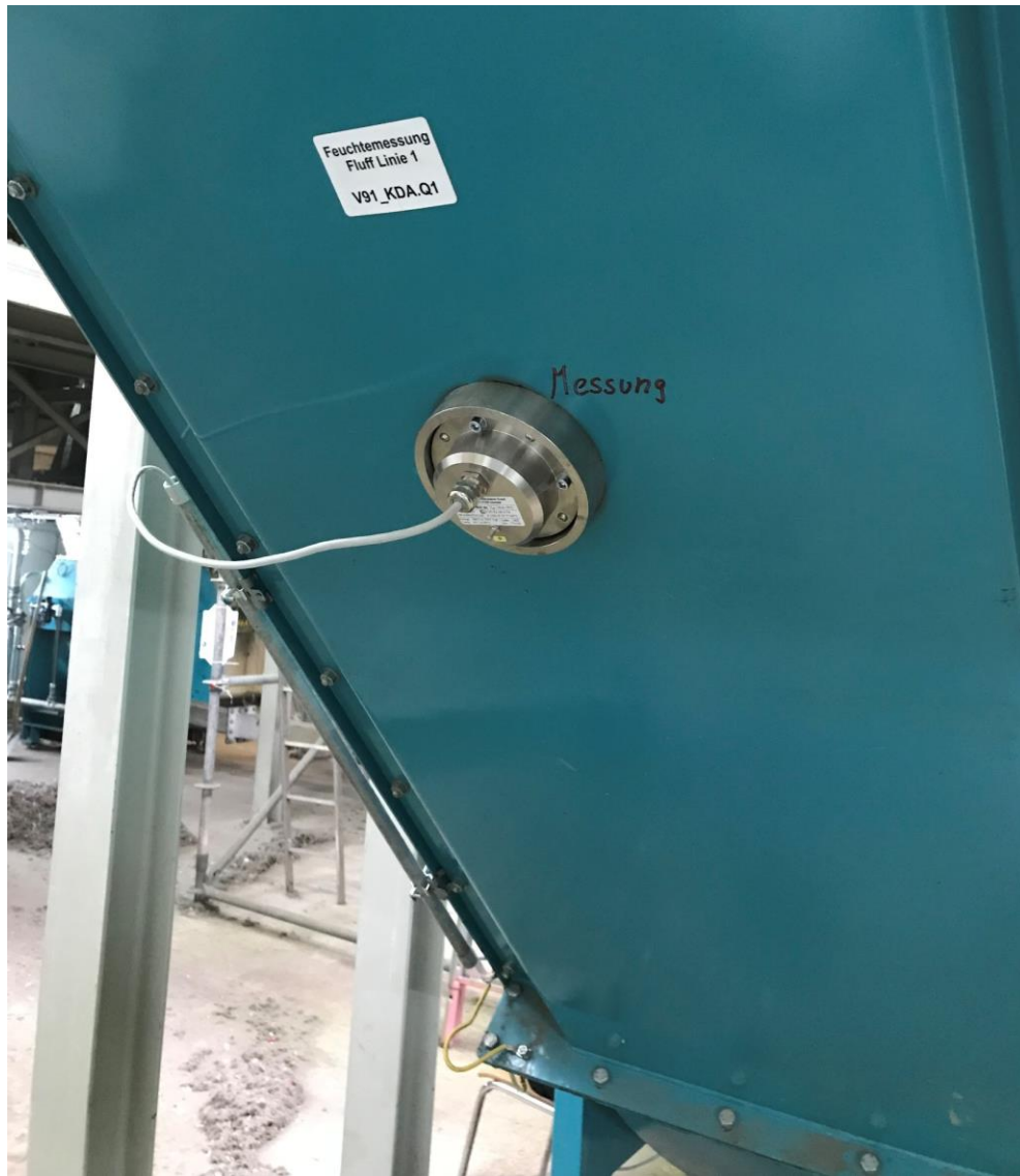
Measurement spot in the conveyor chain before the kiln
